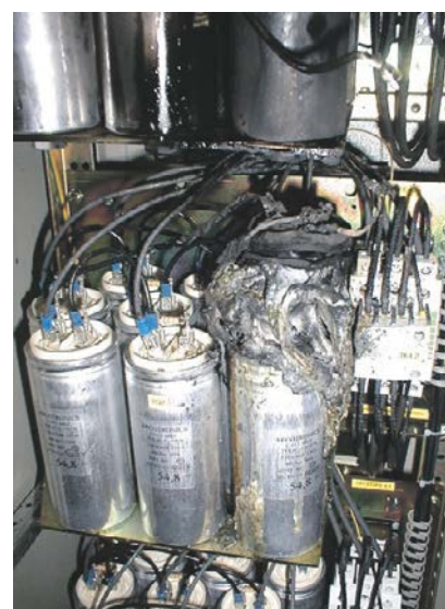
Fig.: Capacitors destroyed by harmonics current
